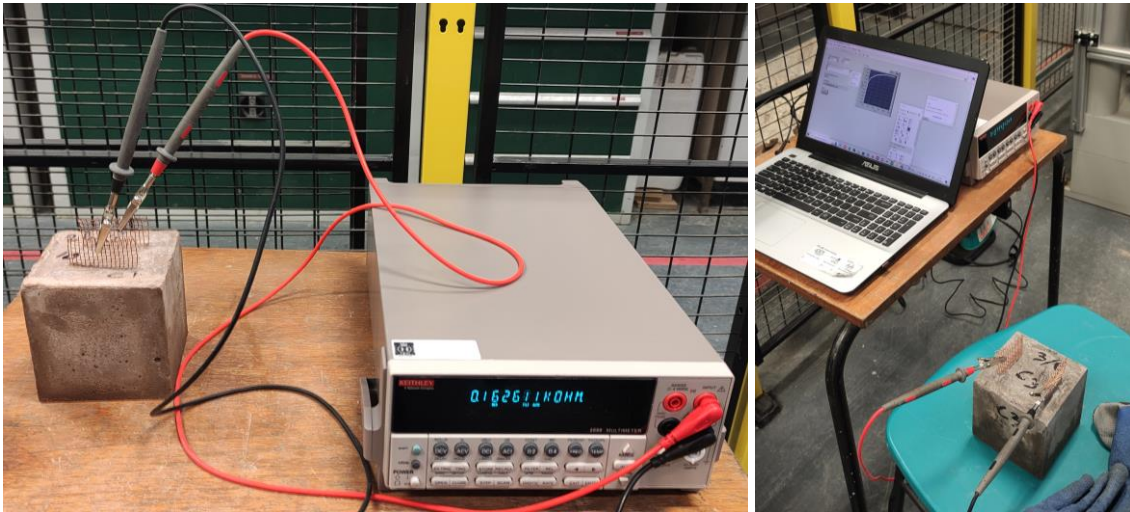
Figure 23 Pre-load data acquisition for self-sensing investigation
