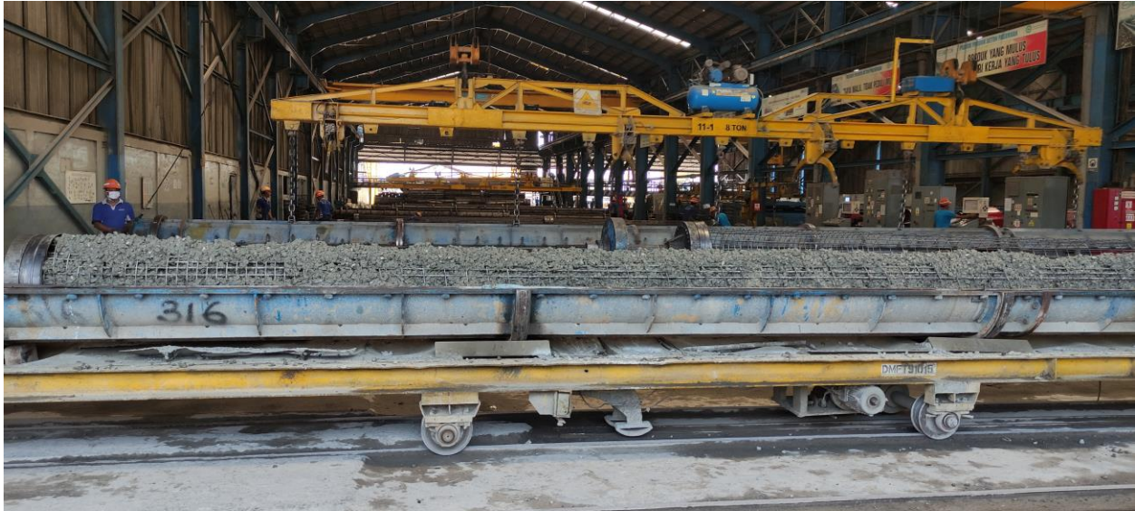
Figure 31 Current production of concrete product in PT. WIKA Beton Surabaya which incorporate 15% fly ash
