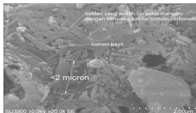
Figure 17 SEM of sample M1000 showing self-healing agent in geopolymer concrete.
