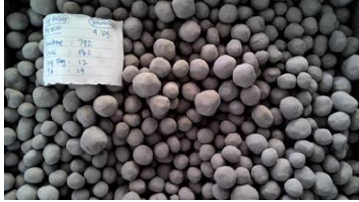
Figure 10: Artificial Aggregate for microbe encapsulation
