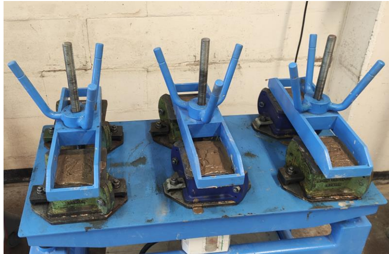
Figure 14 Compacting process for cube sample.
